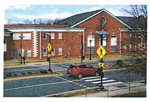
Flashing beacons help improve vehicle compliance with yielding to pedestrians in the crosswalk. This Rectangular Rapid Flashing Beacon (RRFB) is installed in Davidson, NC near a school and busy shopping center.
